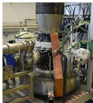
**Gyrotron magnet system operating at Customer's site**
